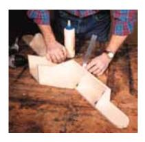
As you assemble the fence, make sure it is square along its length. Be sure and check it again after it is clamped up.
