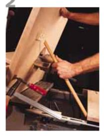
Once the tabletop is hinged to the Workmate's front board, it's easy to locate the the positions for the prop stick and stick bracket.Note the shop-made replacement board for the Workmate top.
